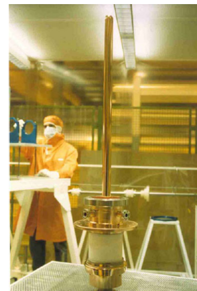
Fig. 5: the 75Ω fixed couplers. Note the two ports for the vacuum gauge and the electron monitor close to the ceramic.
