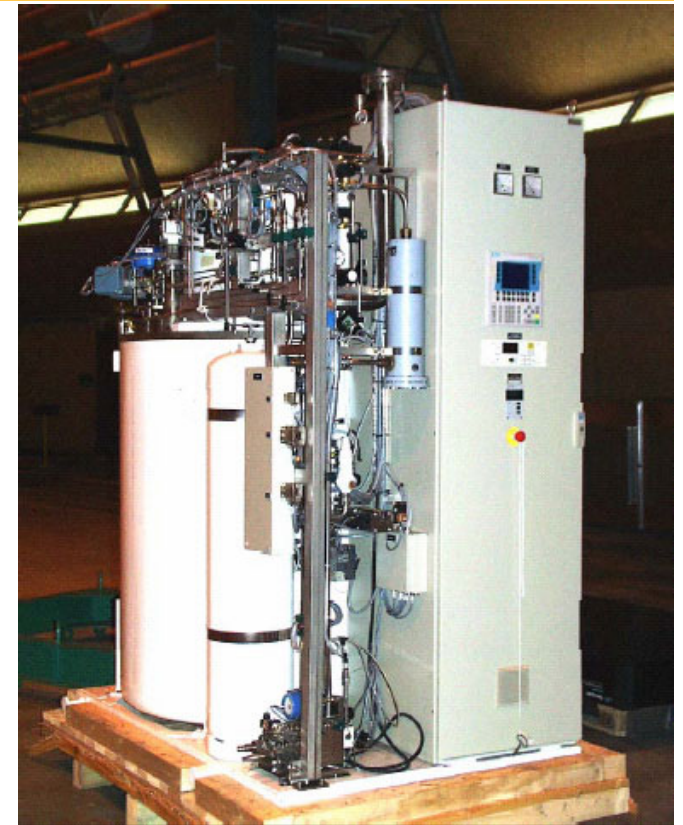
Helial 1000 liquefier/refrigerator 7.5 l/h liquefaction, and 65 W refrigeration at 4.5 K
