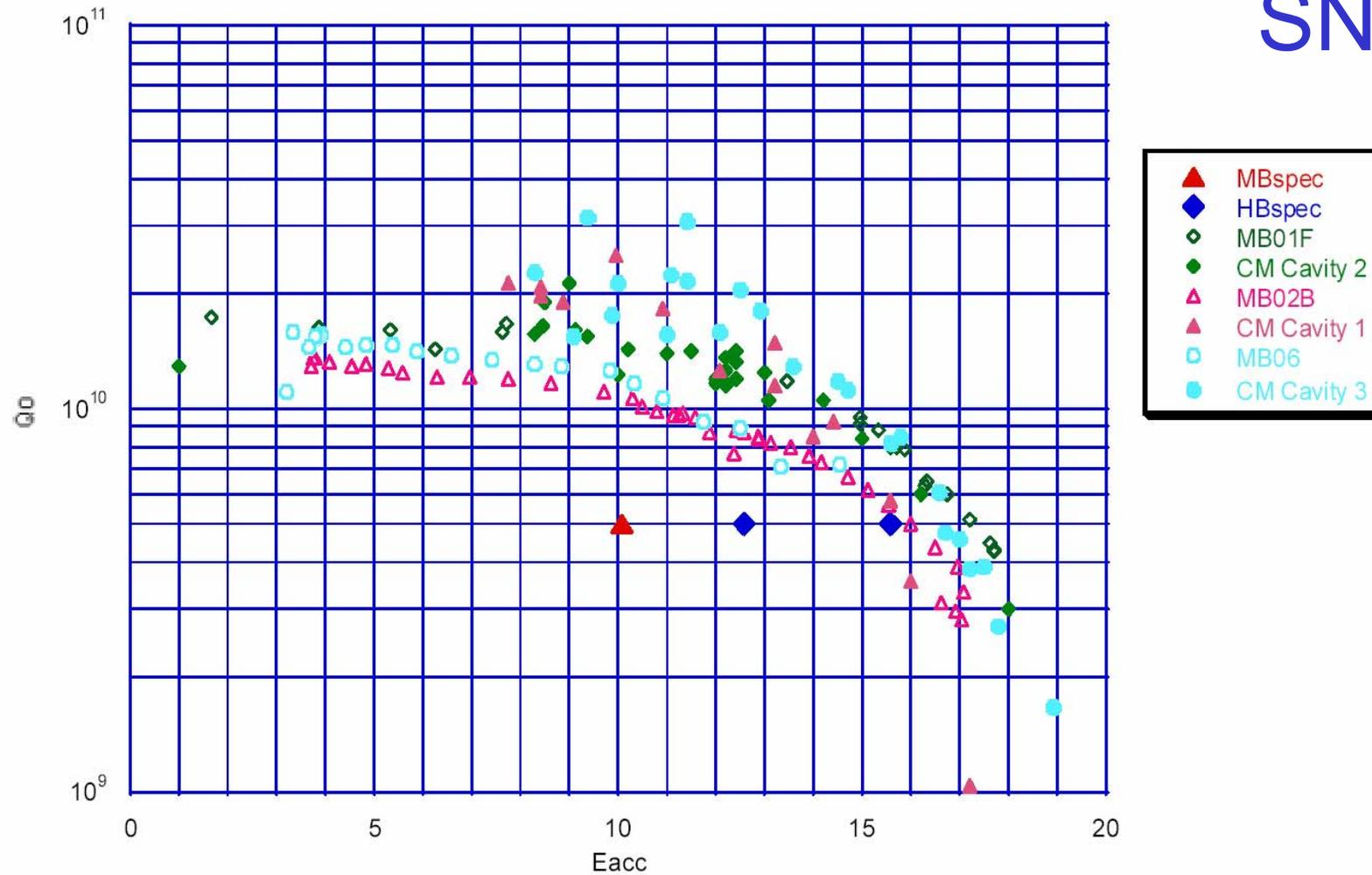
Figure 11. Cavity  $Q_0$  in Final Assembly
