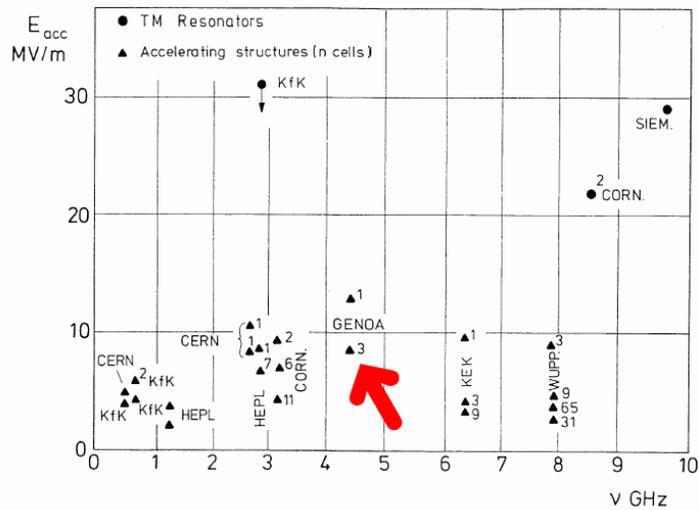
**Accelerating gradient vs. frequency**
