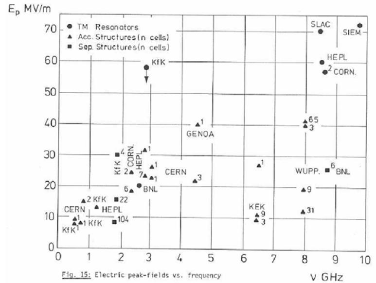
Fig. 15: Electric peak-fields vs. frequency
