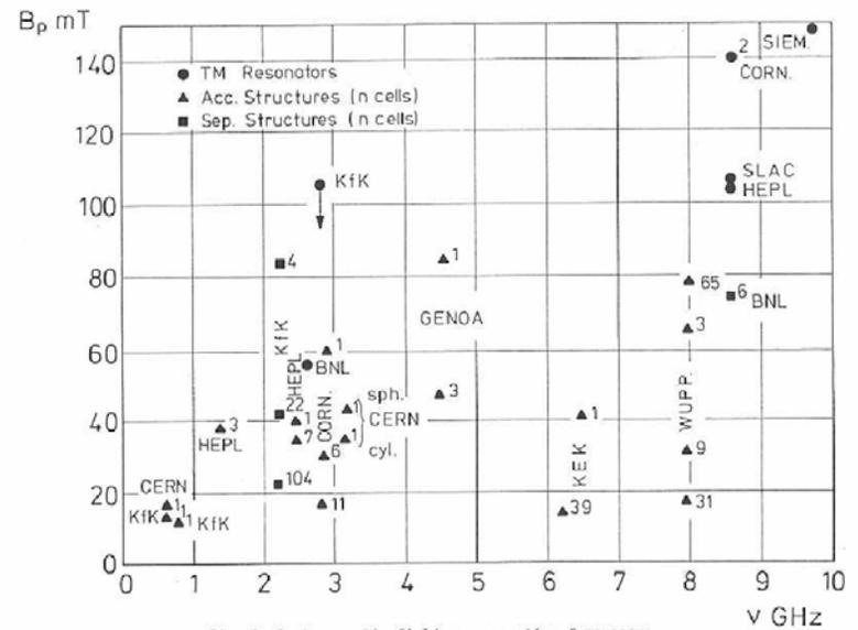
Fig. 1: Peak magnetic field vs. operating frequency
