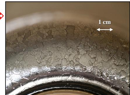
One NbCu clad cavity : 1NC2 ( **BCP + 140°C/30h** )
