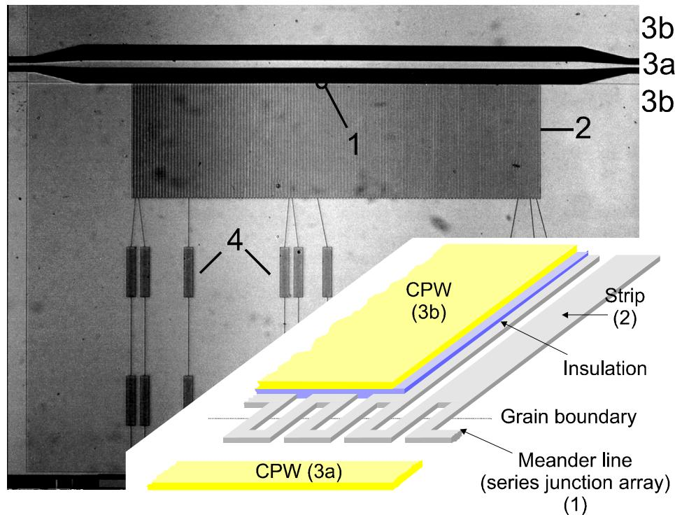
Irradiation of microwaves by a coplanar waveguide
