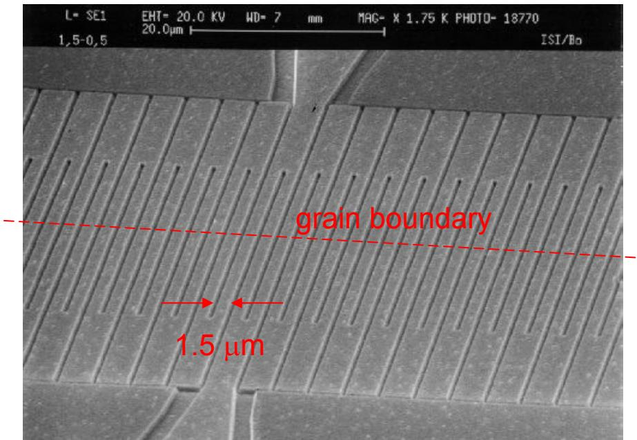
Fabrication of an array of bicrystal junctions by submicrometer lithography
