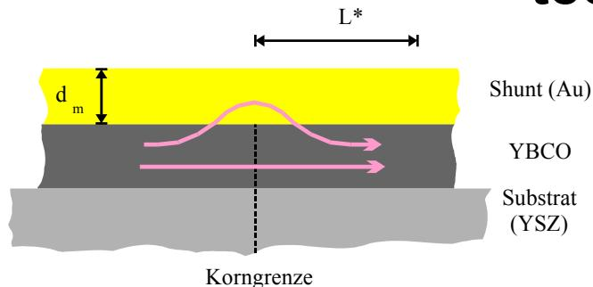
YBCO bicrystal junction with in-situ gold shunt : RSJ like I/V characteristic with small (5 %) spread of  $R_n$
