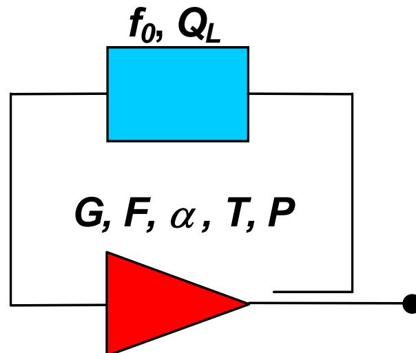
$$L_{osc} = 10 \cdot \log \left[ 1 + \frac{f_0^2}{4Q_L^2 f_m^2} \right] + 10 \cdot \log \left[ \frac{\alpha}{f_m} + \frac{GFkT}{P} \right]$$
