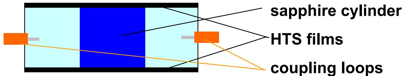
**$Q \approx 10^5 - 10^6$ :** attractive for surface impedance measurements of HTS films and low phase noise oscillators (5 to 30 GHz)
