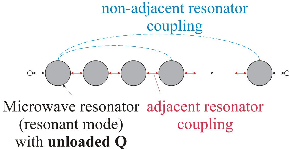
**coupling only between adjacent resonators  $\Rightarrow$  Chebyshev-type characteristic**
