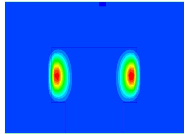
$Q \approx 10^6 - 10^7$ : very attractive for mm wave low-phase noise oscillators (10 to 70 GHz)
