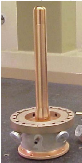
Figure 12. The SNS coupler is based on a modification of the KEK-B coupler. The window matching design has
