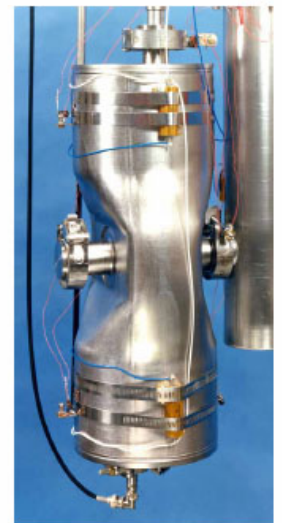
Figure 7: Concept and realization of a 350 MHz, \beta=0.12 coaxial half-wave resonator [2,23].
