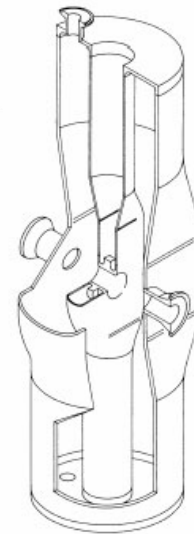
Figure 7: Concept and realization of a 350 MHz, \beta=0.12 coaxial half-wave resonator [2,23].
