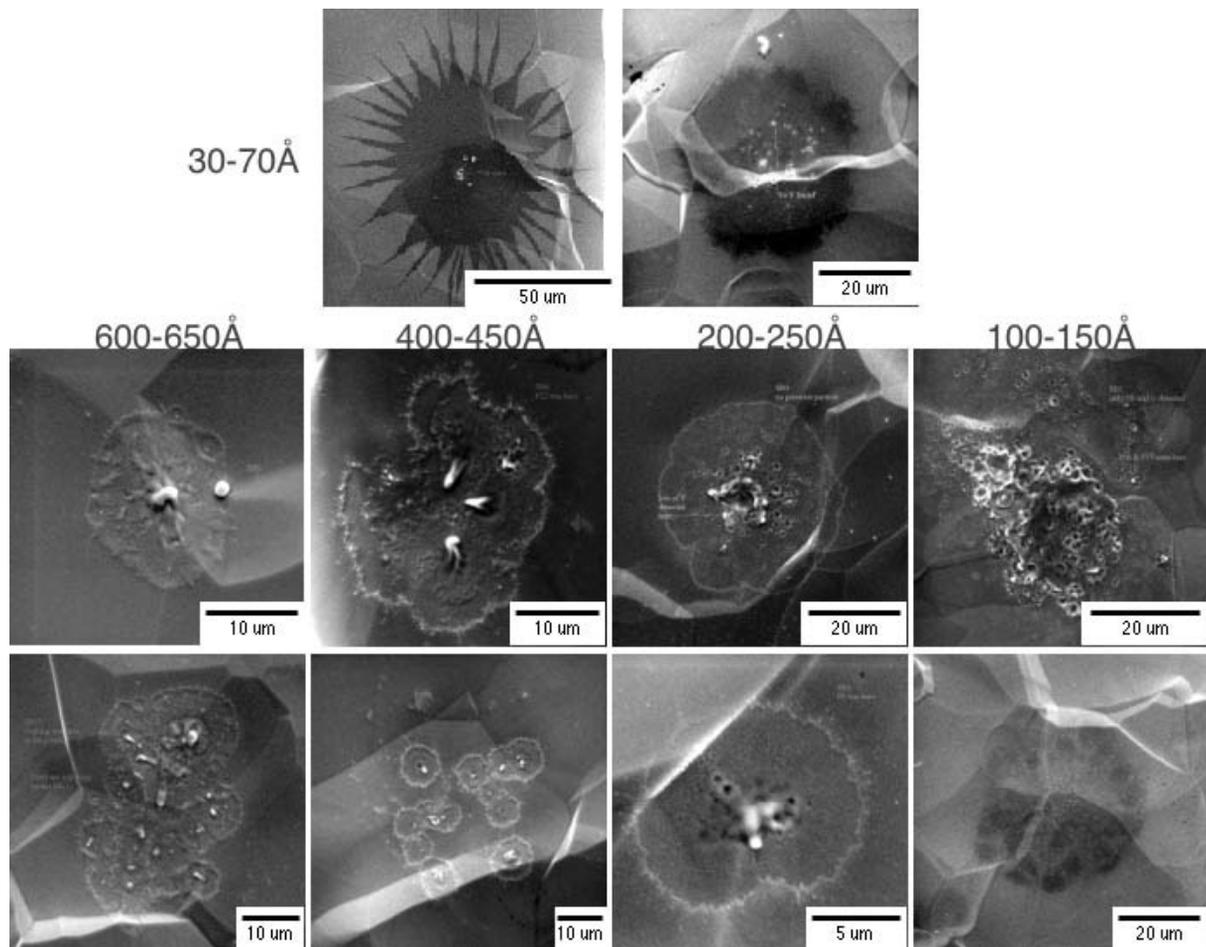
Figure 1: Starbursts (*i.e.*, regions of intense ion bombardment during breakdown) on niobium with varying oxide thickness. The natural oxide on niobium is usually about 30–60Å. The top left picture displays the characteristic pattern that suggested the name “starburst.”
