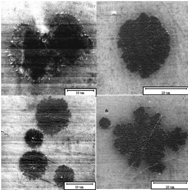
Figure 3: Starbursts on heavily oxidized copper (note similarity to starburst on heavily oxidized niobium)
