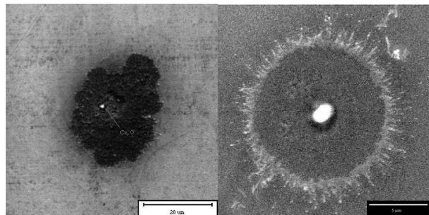
Figure 2: Typical starbursts on copper (left) and niobium (right) with thick oxides (The micron bar for the left picture is 20 $\mu$ m long, and that for the right picture is 5 $\mu$ m long.)
