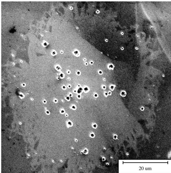
Figure 4: A typical starburst on gold (1000Å gold film sputtered on a niobium substrate) shows heavy cratering all over the starburst region; gold has a very thin oxide.
