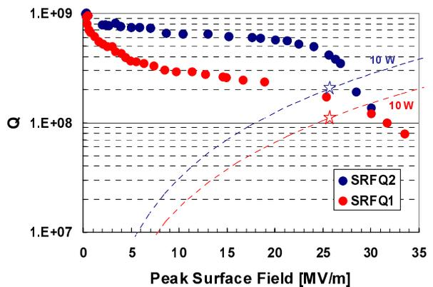
Figure 2: Q-curves of SRFQ1 and SRFQ2 exceed the design specifications (25.5 MV/m at 10 W)
