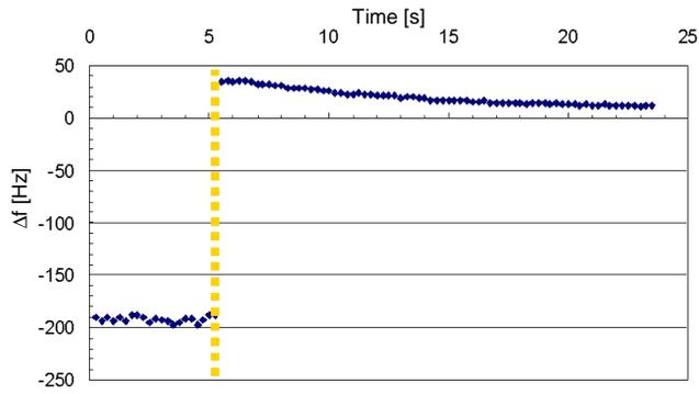
Figure 10: Typical frequency change induced in the SRFQ1 resonator by a heavy hammer stroke on the test cryostat outer vessel: however, no vibrations seem to have been induced (the resolution is 250 ms).
