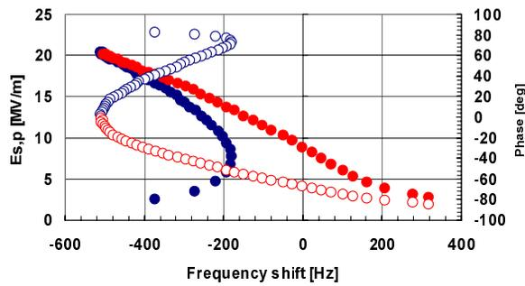
Figure 6: Folded resonance curves of the Lorenz detuned resonators: blue bullets correspond to the stable part of the curve, red bullets to the unstable one.
