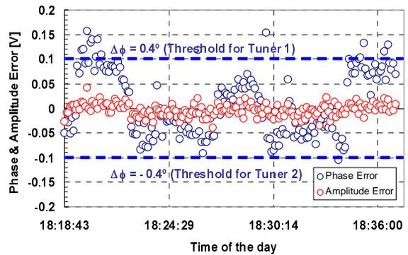
Figure 8: Typical excursions of phase and amplitude errors in the SRFQ’s in the test cryostat: the phase error values, at which the mechanical slow tuners are moved, are shown.
