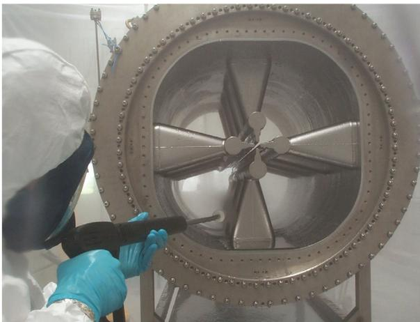
Figure 1: SRFQ1 during high pressure water rinsing, before being assembled into the final cryostat.
