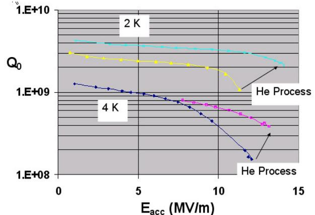
Figure 5: Test results for the LANL  $\beta=0.175$ , 2-gap spoke resonator.
