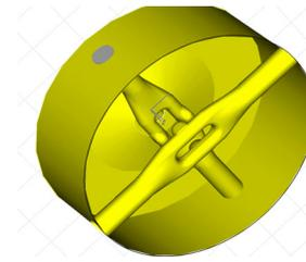
Figure 7: A LANL designed  $\beta=0.125$  3-gap spoke resonator with RF-focusing in the center-gap.
