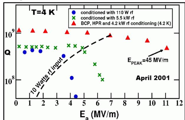
Figure 4: 4.2 K test results for the ANL  $\beta=0.4$ , 2-gap spoke resonator.
