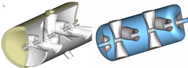
Figure 6: An ANL 4-gap spoke resonator at  $\beta=0.62$  (left) and a 5-gap,  $\beta=0.48$  spoke resonator from LANL. Both are investigated for their potential to replace similar elliptical resonators.
