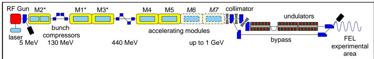
Figure 3: Schematic overview of the TTF linac phase 2 (not to scale). Beam direction is from left to right, the total length is 250 m.
