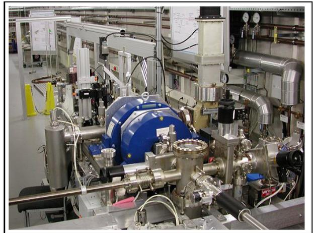
Figure 5: RF gun during the tests at PITZ in DESY-Zeuthen. In the front the cathode load lock system. The RF gun is inside the solenoids (blue).
