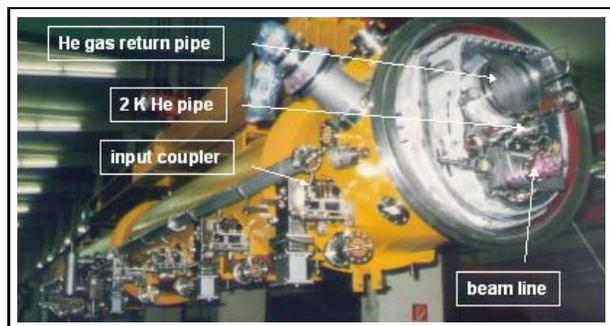
Figure 1: Third generation TESLA superconducting acceleration module during assembly.
