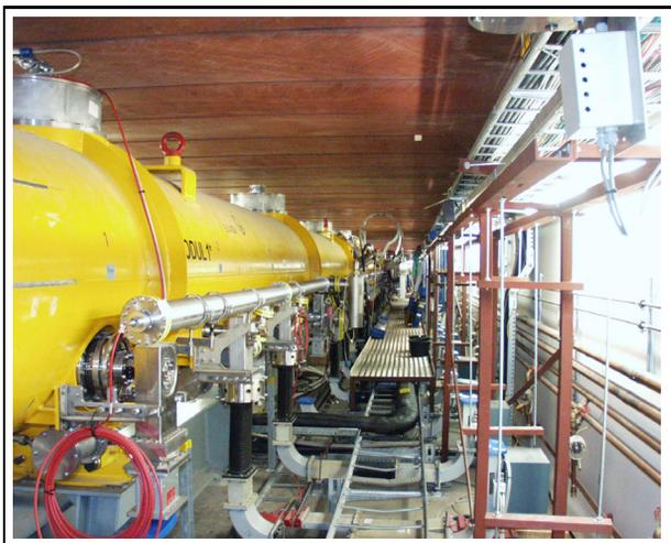
Figure 4: Superconducting TESLA modules installed in the TTF linac during installation of the waveguides.
