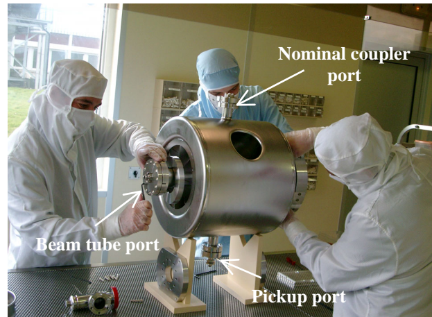
Figure 9: Final assembly of the cavity into the clean room (class 100). Note: in this case, the antenna was attached to the beam port.
