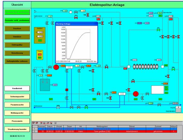
Figure 5: Main window of the visualization.
