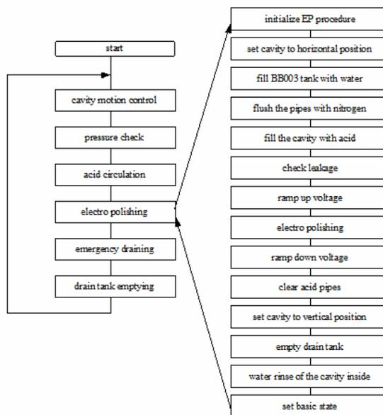
Figure 2: Procedures and sequences of the process [2].
