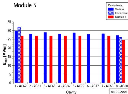
Figure 7: Cavity performance of module 5 at DESY
