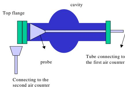
Figure 1: Sketch of particle measurement system
