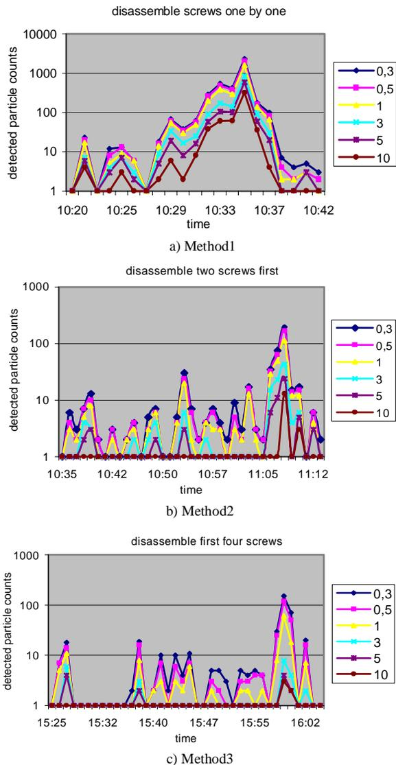
Figure 3: Three disassembly methods without Ar flow
