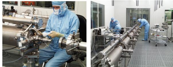
Figure 6: Cavity assembly in clean room
