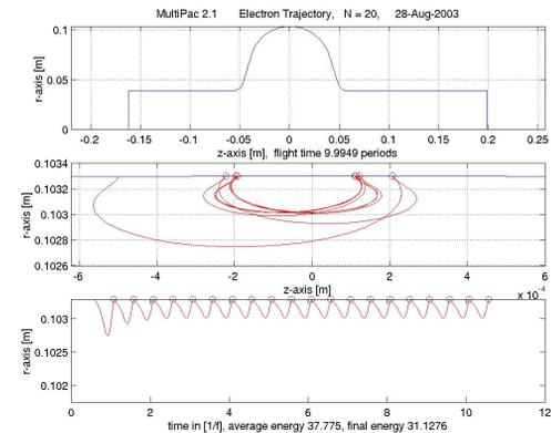
b) Electron trajectory when  $E_p$  is 42.5 MV/m (similar to that of the Tesla middle cell)
