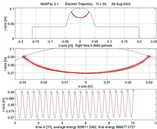
Figure 5: mesh size=6mm, field step size=100kV/m, at Ep=61.5MV/m, the final energy Ef=890keV.
