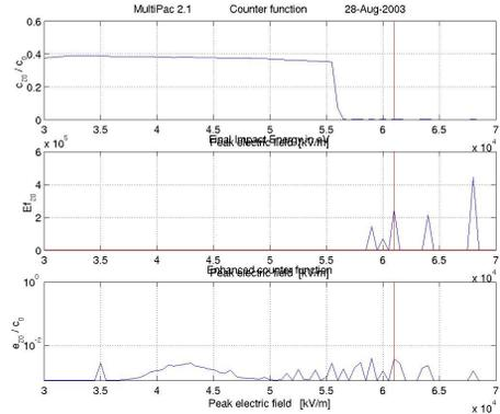
a) Zoomed from Figure 3a,  $E_p$  is from 30-70 MV/m, field step is 500 kV/m
