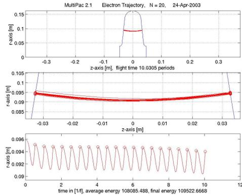
b) Electron trajectory at Ep=6.1MV/m, final energy is 110keV
