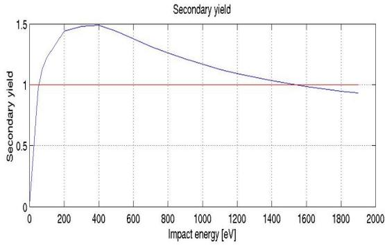
Figure 2: The secondary electron yield at different impact energies (in eV) for a niobium surface baked at 300°C.
