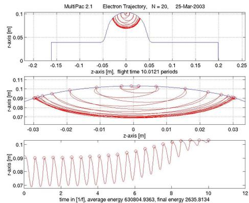
b) Electron trajectory at  $E_p=60$  MV/m, final energy  $E_f=2.6$  keV
