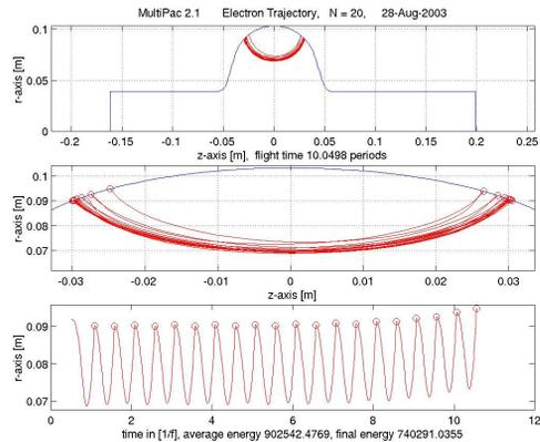
c) Electron trajectory at  $E_p=61$  MV/m, final energy  $E_f=740$  keV
