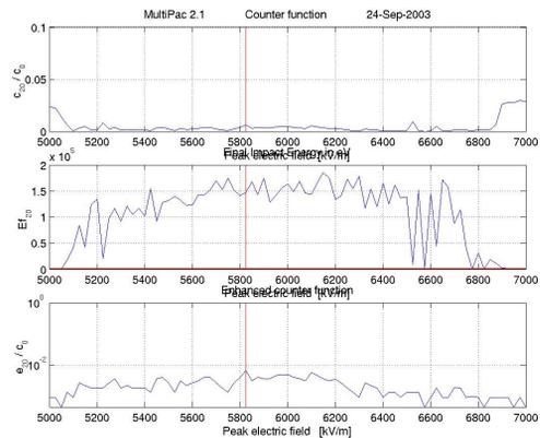
c) Zoomed from a) Ep is from 5-7MV/m, field step is 25kV/m
