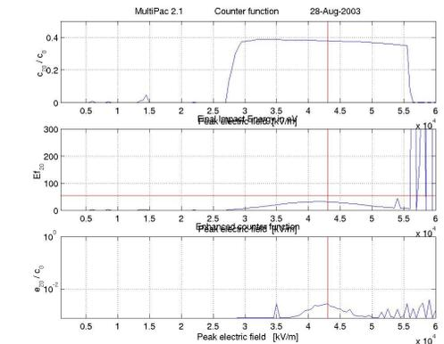
a)  $E_p$  is from 1-60 MV/m and field step is 500 kV/m
