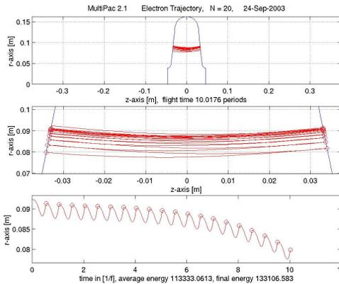
d) Electron trajectory at Ep=5.8MV/m, final energy is 133keV
