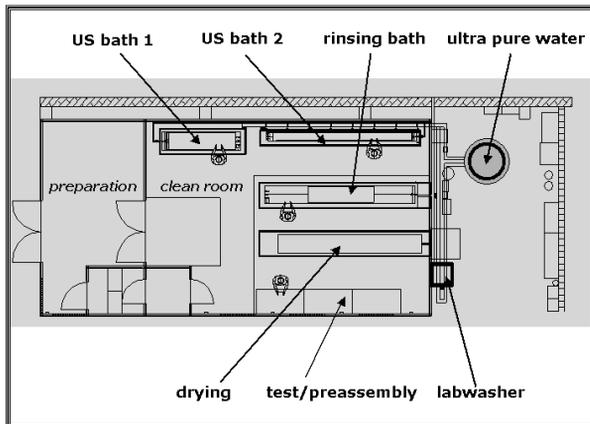
Figure 1: Floor plan of the cleaning facility.
