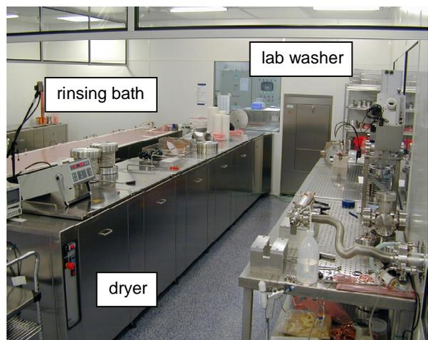
Figure 2: Inside the cleaning facility: rinsing bath and dryer on the left, access to the dish washer in the middle and preassembly bench on the right.
