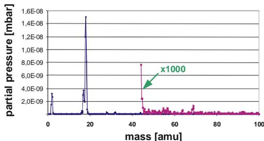
Figure 4: Residual gas spectrum of a cleaned mirror chamber. The intensities for masses larger 44 are enlarged by a factor of 1000.
