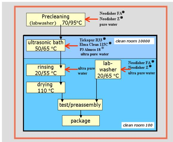
Figure 3: Process chart of the cleaning process.
