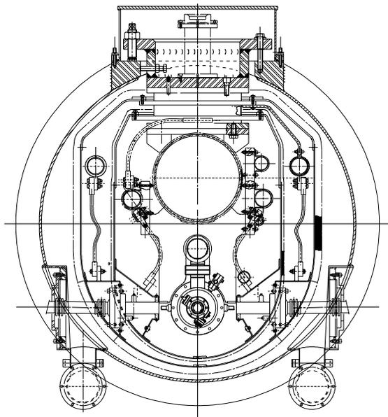
Figure 19: Cryostat/Coldmass cross-section.
