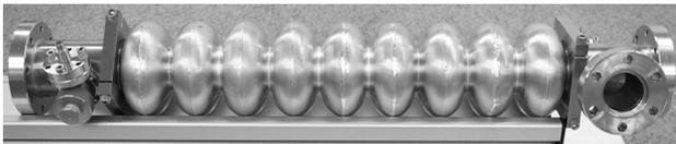
Figure 6: Copper cavity prototype.
