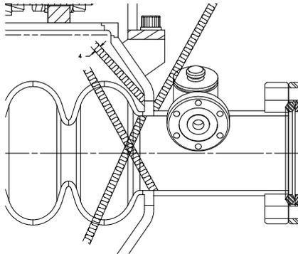
Figure 10: E-beam welding angles.
