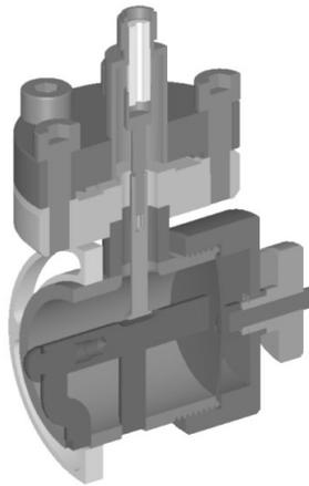
Figure 5: Section view of HOM Coupler.
