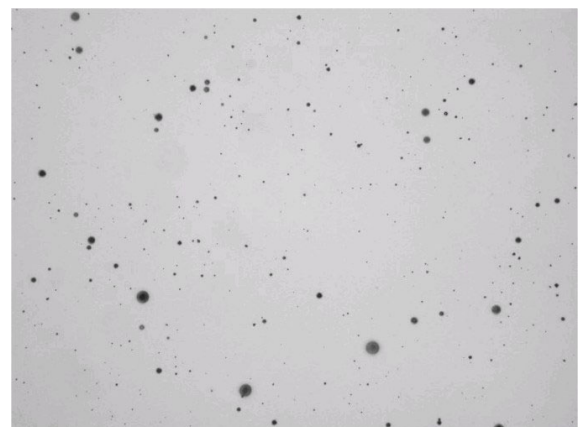
Figure 7: An optical image of the niobium film surface used for microdroplet analysis. Microdroplets show up as dark spots.
