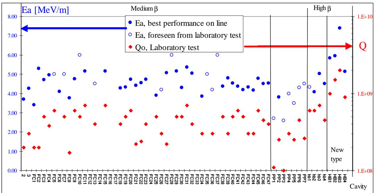
Figure 2: Performance of produced and measured sputtered resonators; the highest  $Q_0$  and accelerating field values have been obtained in properly built substrates. Average operational accelerating field is now 6 MV/m for high  $\beta$  new type resonators; 4.4 MV/m for medium  $\beta$  cavities.
