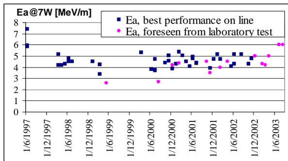
Figure 1: Performance of QWR Nb sputtered resonators as measured on line (blue squares) or in laboratory (pink circles) when not yet measured on line.
