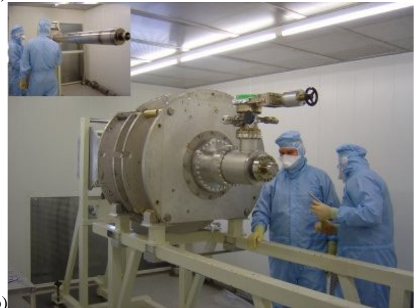
Figure 9: Design of a CH mode cavity under production at ACCEL for Universität Frankfurt. Parts out of copper for testing of production procedures are produced by deepdrawing already. Production of niobium parts has started.
