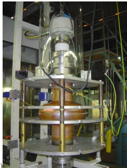
Figure 10: 500 MHz cavity for Cornell University a) in the chemical plant receiving surface preparation for sputtering, b) in the clean room during liner assembly, c) on the sputter apparatus.
