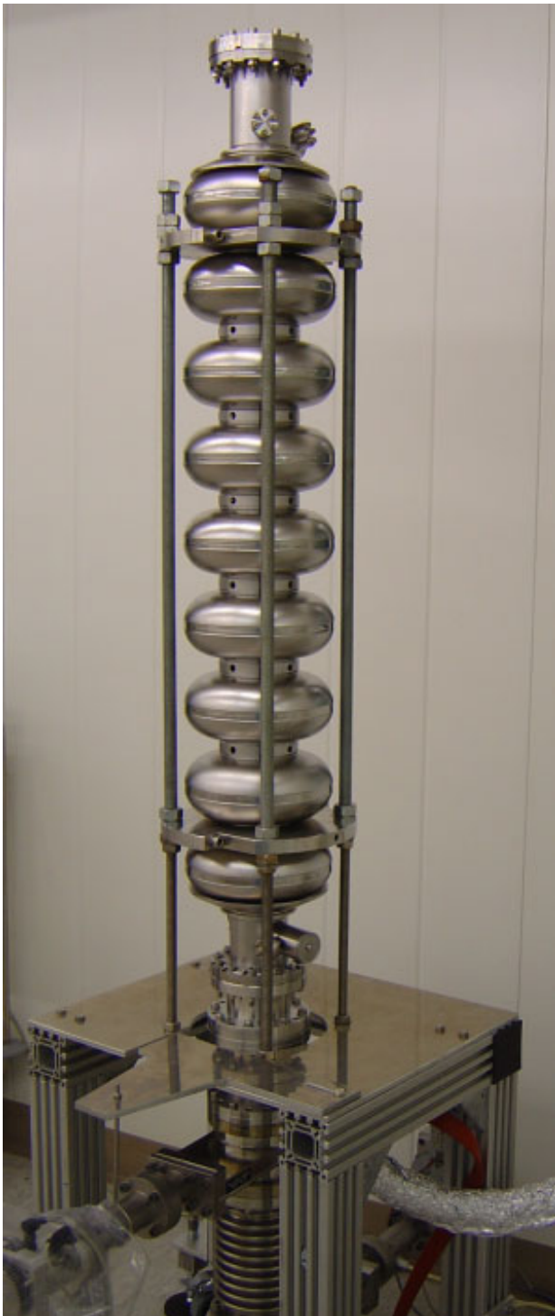
Figure 6: TESLA cavity for BESSY mounted on the new high pressure rinsing system inside the clean room.
