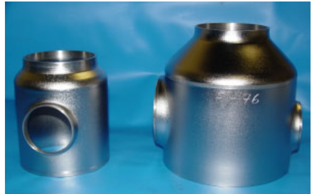
Figure 1: Raw end groups produced for SNS cavities by deep drawing and nipple pulling from one sheet.
