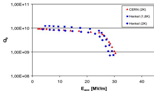
Figure 4: Test of a welded cavity after CERN EP and Henkel EP. The tests were done before in-situ bake. The typical Q-slope can be seen.
