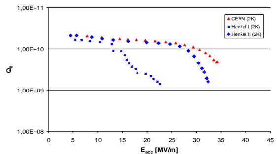
Figure 5: Behaviour of the spun cavity after in-situ bake. The CERN test shows good performance of 35 MV/m. The first test after EP at Henkel was suffering from strong field emission due to problem during the baking preparation at DESY. A new high pressure rinsing improved the performance to fields above 32 MV/m.
