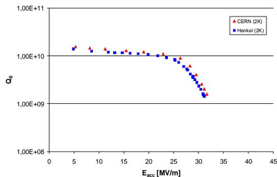
Figure 3: Test of the spun cavity after CERN EP and Henkel EP. The tests were done before in-situ bake. The typical Q-slope can be seen.
