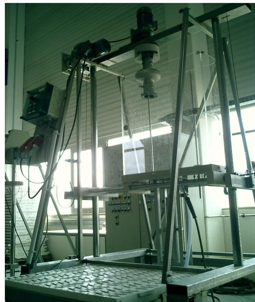
Figure 2: Setup to rinse cavity with diluted nitric acid and ultrapure water
