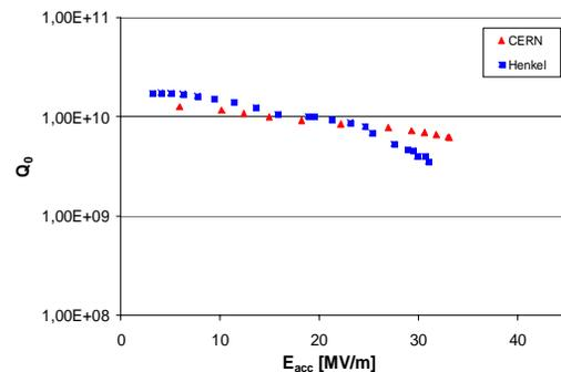
Figure 6: Behaviour of welded cavity after in-situ bake. The CERN test shows good performance of 33 MV/m. The first test after EP at Henkel was suffering from a vacuum leak. The cavity degradation starting at 20 MV/m is due to this problem. The maximum gradient is 31 MV/m. A new test is under preparation.
