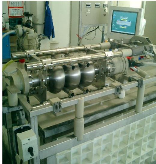
Figure 1: Setup for electropolishing
