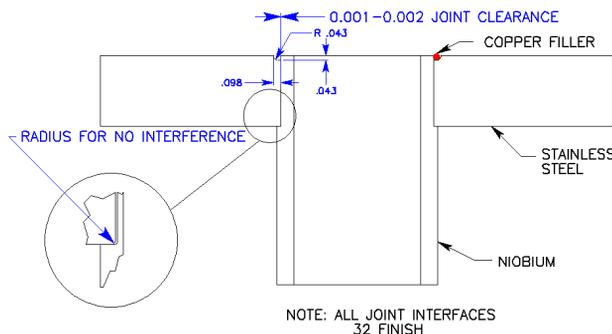
Figure 1: Braze joint configuration.
