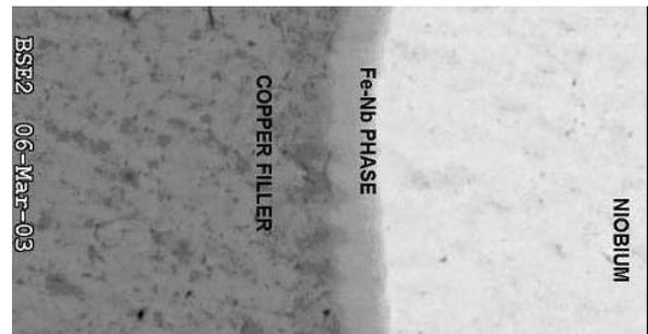
Figure 7: SEM closeup of copper/niobium transition.
