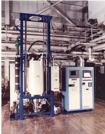
Figure 2: ANL hydrogen/vacuum furnace.
