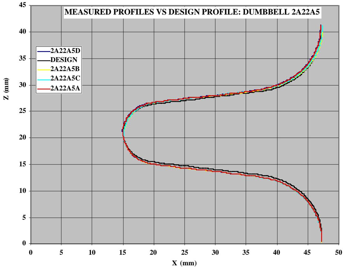
Figure 6: Measured profiles compared to design profile
