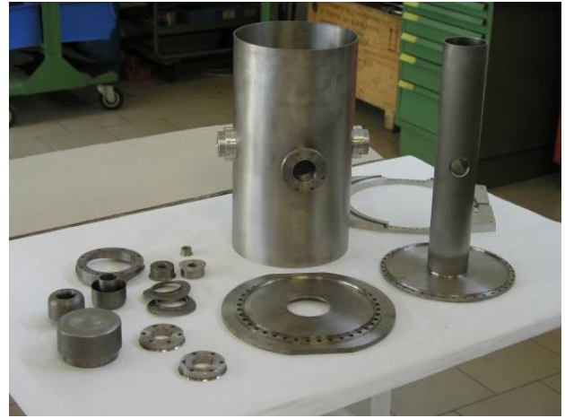
Figure 3: Resonator parts before welding.
