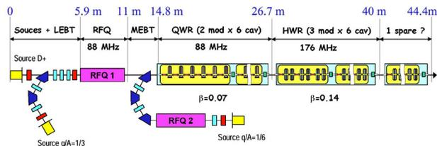
Figure 1: Architecture of the Spiral-2 driver linac.
