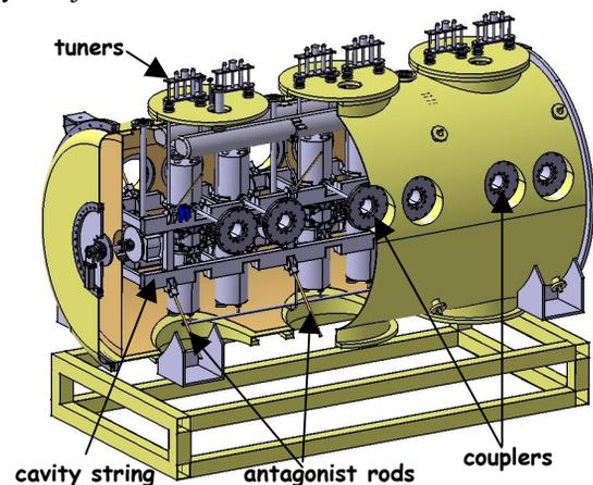
Figure 10: HWR cryomodule.
