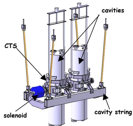
Figure 9: HWR cavity string.
