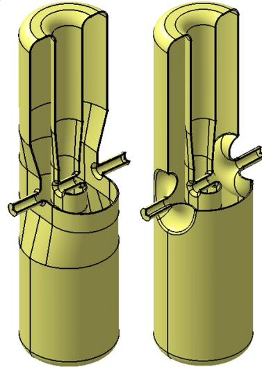
Figure 4: “Juelich-type” (left) and “Argonne-type” (right) HWR models.
