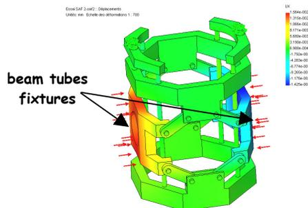
Figure 8: HWR cold tuning system.
