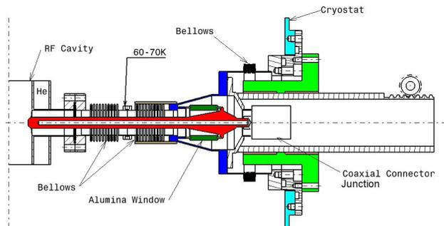
Figure 7: Coupler structure (courtesy of LPSC Grenoble).
