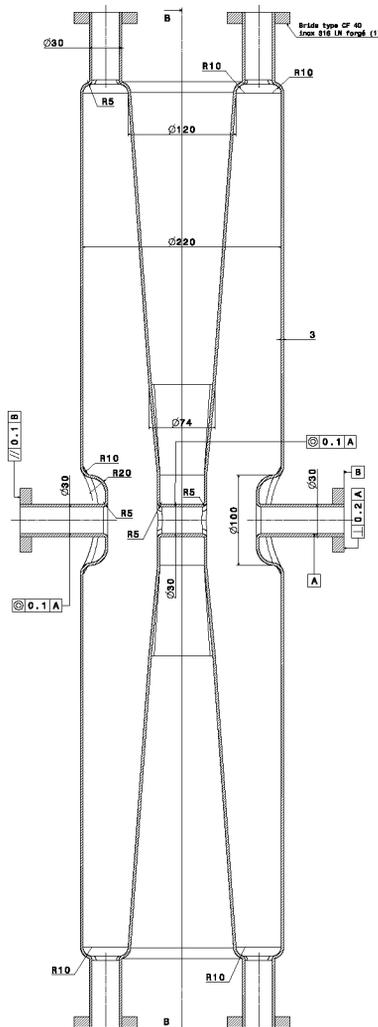
Figure 6: Vertical cut view of the final HWR prototype.
