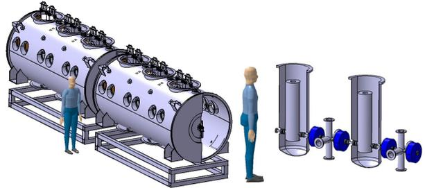
Figure 12 (left): View of two subsequent cryomodules in the reference design using SC solenoids.
