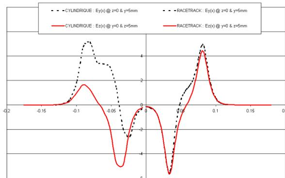
Figure 3: Transverse electric fields  $E_y$  (black dot curve) and  $E_z$  (red curve) along the x beam axis (5 mm off axis). Left: cylindrical shape. Right: racetrack shape.
