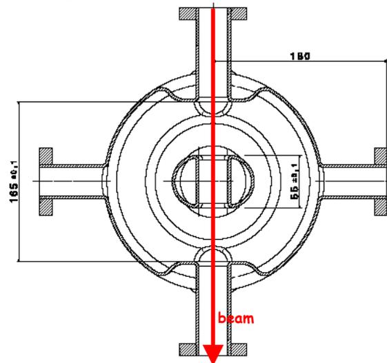
Figure 5: Horizontal cut view of the final HWR prototype in the beam axis region.
