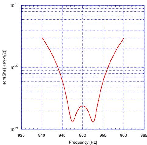
Figure 12: Calculated system sensitivity ( $\omega_m \sim \omega_2 - \omega_1 \sim 1$  kHz,  $Q = 10^{10}$ ,  $Q_m = 10^6$ ,  $T = 1.8$  K,  $T_{eq} = 1$  K, stored energy  $U \sim 1$  J per cavity)
