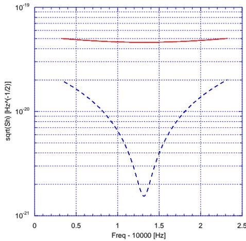
Figure 11: Calculated system sensitivity ( $\omega_m \sim 4$  kHz,  $\omega_2 - \omega_1 \sim 10$  kHz,  $Q = 10^{10}$ ,  $T = 1.8$  K,  $T_{eq} = 1$  K, stored energy  $U \sim 10$  J per cavity and a)  $Q_m = 10^3$  (solid line); b)  $Q_m = 10^6$  (dashed line))
