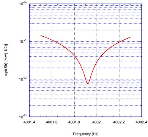
Figure 13: Calculated system sensitivity ( $\omega_m \sim 1$  kHz,  $\omega_2 - \omega_1 \sim 4$  kHz,  $Q = 10^{10}$ ,  $Q_m = 10^6$ ,  $T = 1.8$  K,  $T_{eq} = 1$  K, stored energy  $U \sim 1200$  J per cavity)
