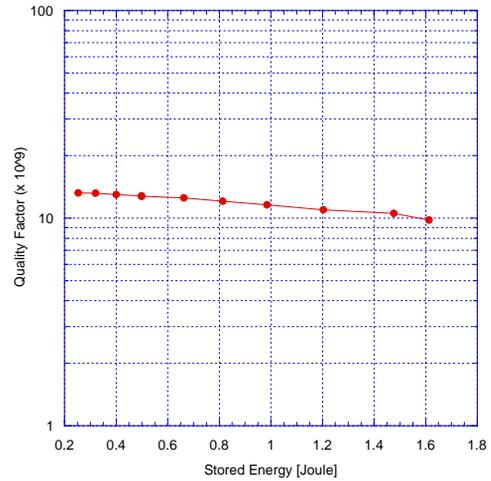
Figure 7: Quality factor vs. stored energy for the fixed-coupling cavity of Fig. 2
