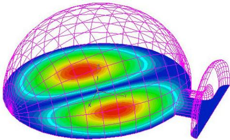
Figure 5: Electric field magnitude of the  $TE_{011}$  mode. Note the alignment of the field axis
