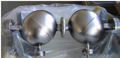
Figure 3: Niobium spherical cavities (variable coupling)
