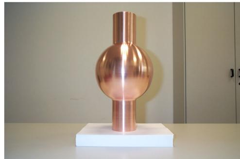
Figure 8: Single-cell, seamless, copper cavity
