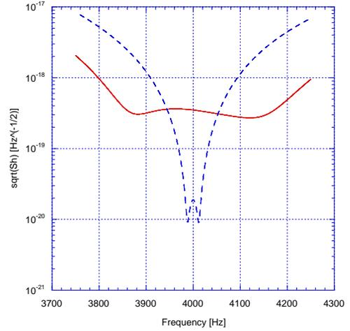
Figure 10: Calculated system sensitivity ( $\omega_m \sim \omega_2 - \omega_1 \sim 4$  kHz,  $Q = 10^{10}$ ,  $T = 1.8$  K,  $T_{eq} = 1$  K, and a)  $Q_m = 10^3$ , stored energy  $U \sim 10$  J per cavity (solid line); b)  $Q_m = 10^6$ , stored energy  $U \sim 0.1$  J per cavity (dashed line))
