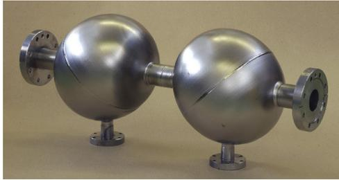
Figure 2: Niobium spherical cavities (fixed coupling)
