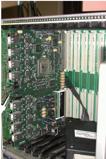
Fig.10: Digital signal processor board with 8 Gigalink interfaces for fast analog and digital IO.
