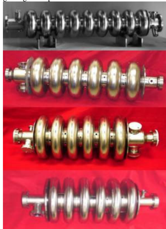
Figure 1: Bulk niobium cavities for various particle velocities. From top: a) TESLA niobium 9-cell cavity for \beta=1 . b) SNS six-cell for \beta=0.81 . b) SNS six-cell for \beta=0.61 . b) RIA/MSU six-cell for \beta=0.47 .
