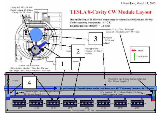
Figure 3: Cross section of the TESLA/BESSY cw module (J.Knobloch,BESSY). The numbers correspond to table 1.
