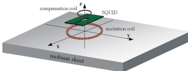
Figure 1: Principle of eddy current measurements with a SQUID.
