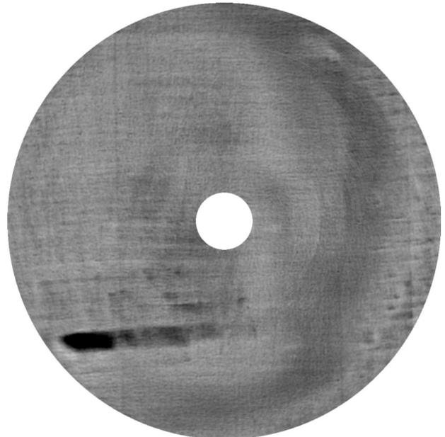
Figure 8: Scan of sheet 9 with conventional sensor system. The y-val. of channel 1 (at 170 kHz) is shown. None of the scratches is visible, as the back of the sheet is far beyond the skin depth (0.12 mm) of the frequency used.
