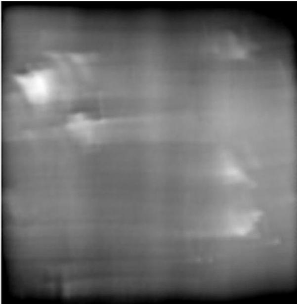
Figure 4: Scan of sheet 41 with SQUID sensor system. Scanning resolution was set to 300 scan lines, which corresponds to 1 l/mm. The frequency used was 33 kHz, which is closer to DESY's measurement channel 1 (170 kHz).
