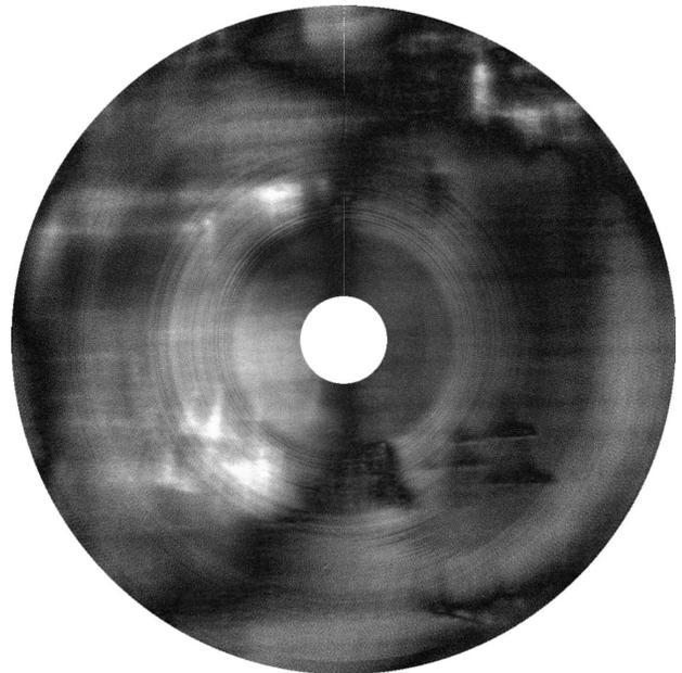
Figure 9: Eddy current scan of sheet 45 (amplitude of channel 1). The dark shapes are partially artifacts caused by lift-off and the signal is close to noise level.
