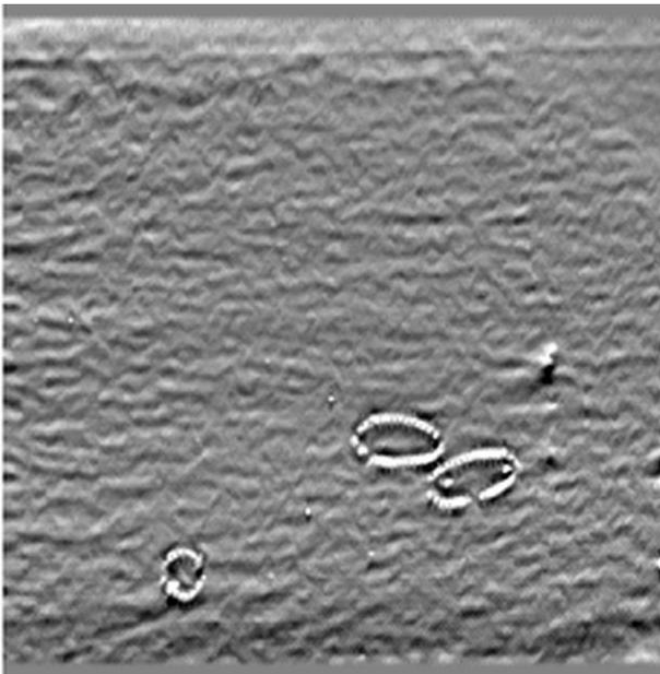
Figure 6: Scan of sheet 9 with SQUID sensor system. The three ellipses shown are pen markings for scratches (within the ellipses) on the BACK of the sheet. Some more dots and one large signal source (center left) are visible.
