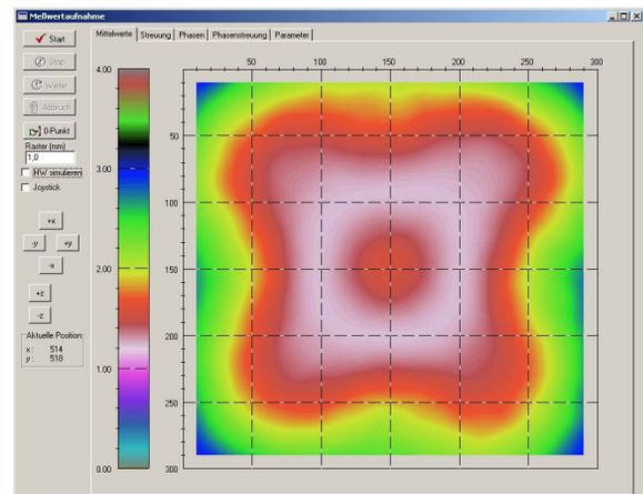
Figure 3: Sample screenshot of the data acquisition software with a simulated surface respond.
