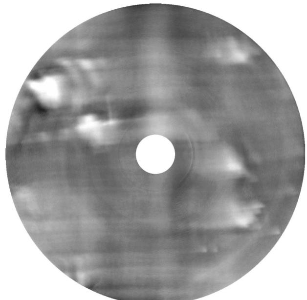
Figure 5: Scan of sheet 41 with conventional sensor system. DESY's default setup was used, with 4.16 l/mm track density. The y-val. of channel 2 (at 1 MHz) is shown, which (in this example) delivers the most similar image).
