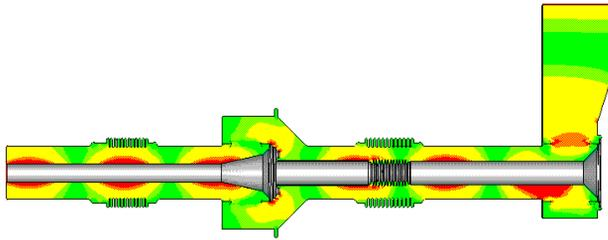
Figure 5: Electric fields in the coupler.
