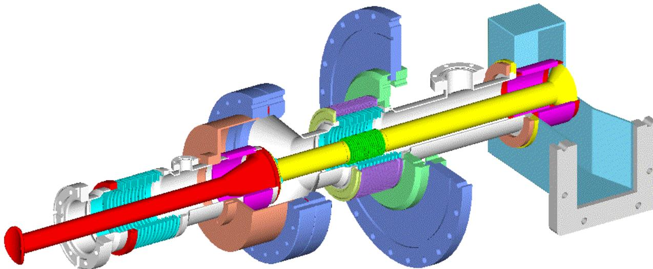
Figure 3: 3D view of the injector cavity coupler.
