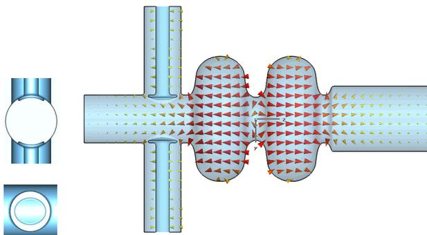
Figure 1: Input coupler in the injector cavity.
