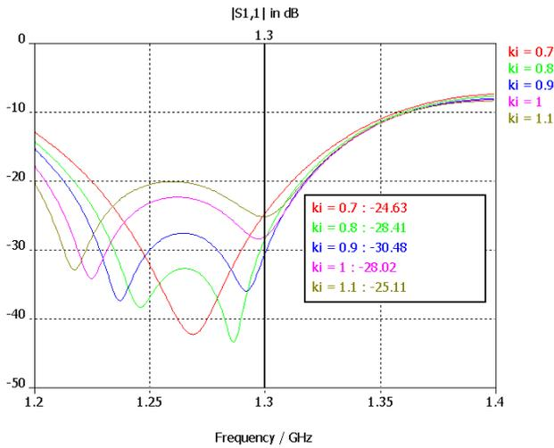
Figure 4: Reflection of the coupler in a frequency range at different coupling (coupling increases from weak to strong when  $k_i$  varies from 0.7 to 1.1).
