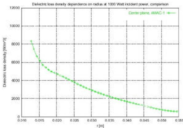
Figure 8a: Radius dependence of dielectric loss at 1000 W incident power for AMAC -1.
