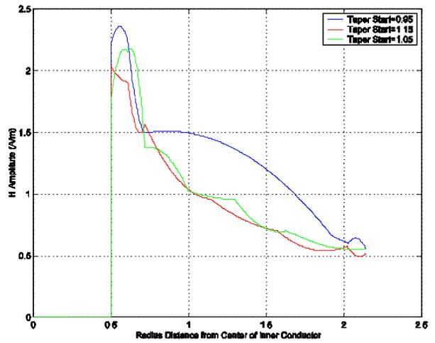
Figure 4: Magnetic Field Amplitude along the Ceramic Window Surface.
