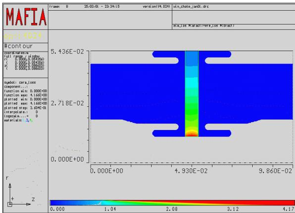
Figure 7: Contour plot of AMAC-1 dielectric losses in the ceramic at  $1/2W$  incident power.
