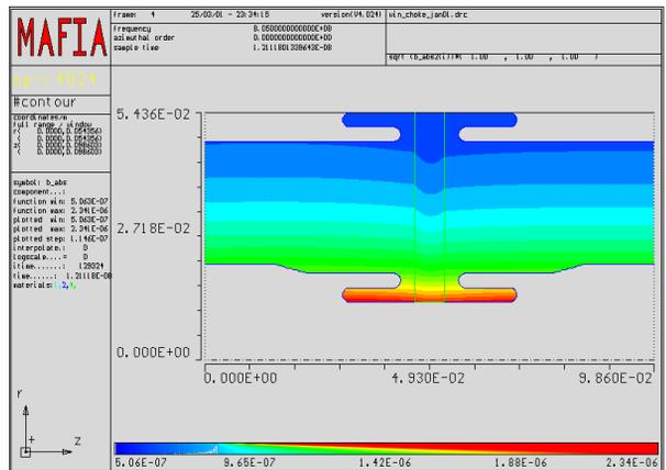
Figure 5: Contour plot of magnetic field in AMAC-1 at 1/2W incident power.
