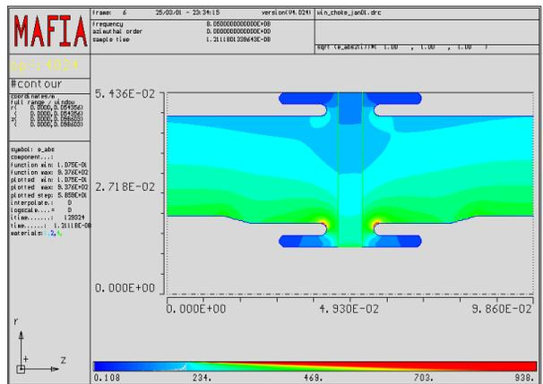
Figure 6: Contour plot of electric field in AMAC-1 at 1/2W incident power.
