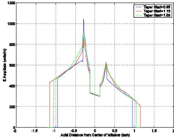
Figure 2: AMAC-1 Electric Field Amplitude along Inner Conductor Surface.
