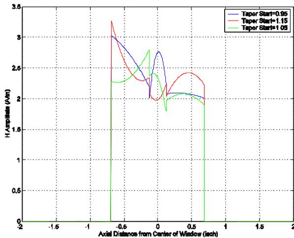
Figure 3: Magnetic Field Amplitude along the Inner Conductor Surface.
