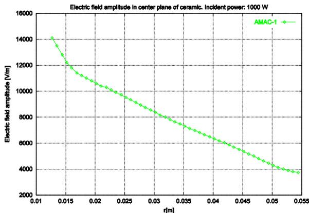
Figure 8b: Radius dependence of electric field at the ceramic center plane of AMAC -1 at 1000 W of incident power.
