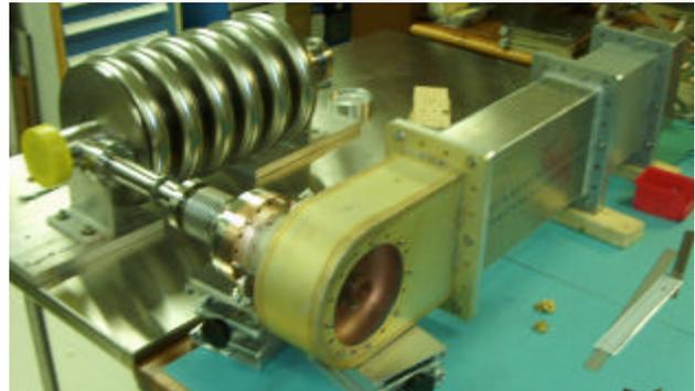
Figure 9: RIA Coupler mounted on SRF Cavity.
