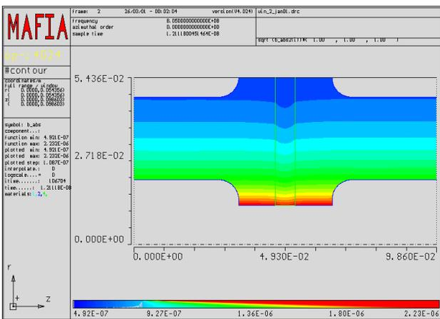
Fig. 4: Contour plot of magnetic field in AMAC-2
