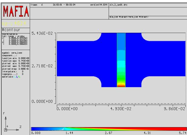
Fig. 5: Contour plot of dielectric loss of ceramic in AMAC-2
