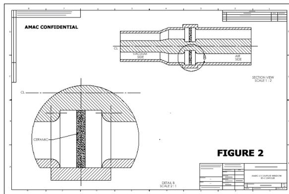
Fig. 2: Window Geometry
