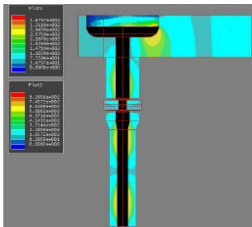
Fig. 1: AMAC-2 Coupler, Electric Fields (V/m for 1W average power)
