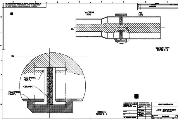
Fig. 8: Window Geometry
