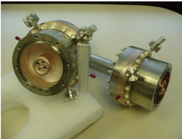
Fig. 3: Coaxial coupler assembly with AMAC-2 (with compression ring) window design
