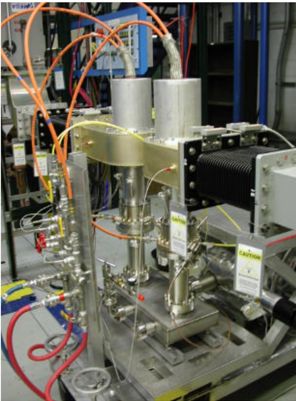
Fig. 10: Jefferson Lab Test Stand with two AMAC windows
