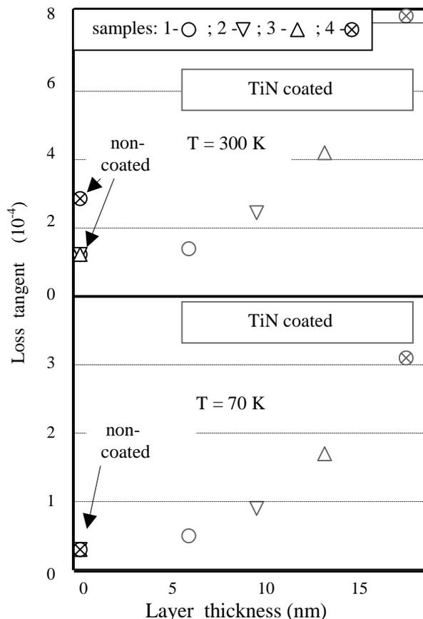
Figure 1: Effective loss tangent for cylindrical “warm” windows of TTF3 coupler as a function of surface TiN layer thickness at 300 K (the top part of the plot) and at 70 K.
