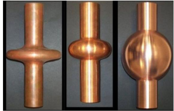
FIG. 2 Three cavities with the same resonant frequency but different beta
