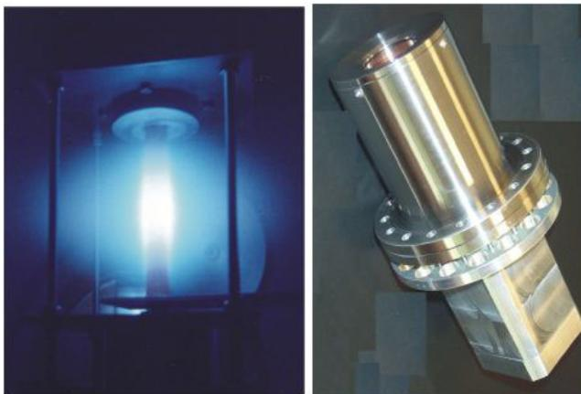
FIG. 7. Cylindrical post-magnetron (left) and 2 inches planar magnetron source (right)
