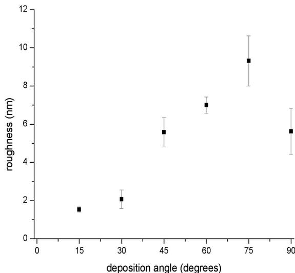
FIG. 12. Calculated average roughness vs. deposition angle
