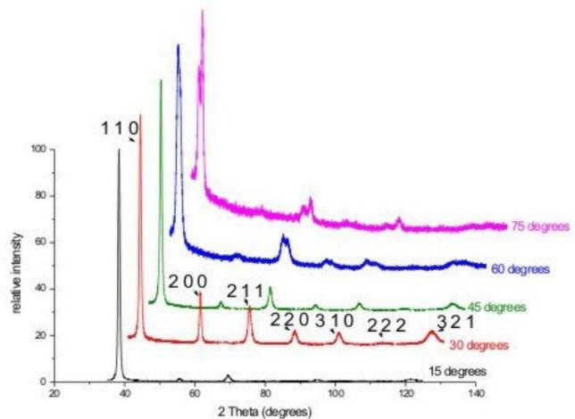
FIG. 10. Normalized X-ray diffraction spectra at various deposition angles
