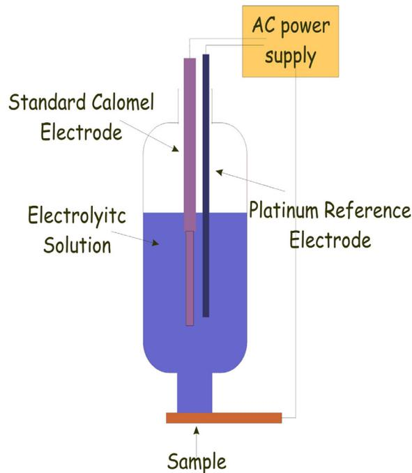
FIG. 13. Schematic view of experimental apparatus for impedance spectroscopy measurement
