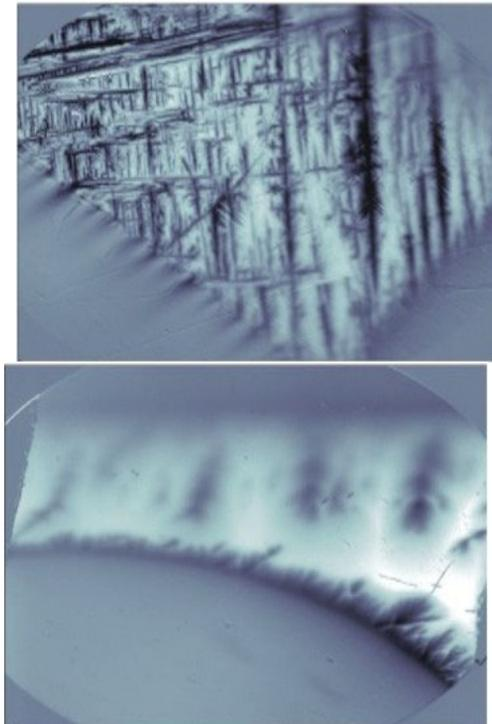
FIG. 16. Magneto-optical images of film deposited at target - substrate angle of 0 (top) and 45 (bottom) degrees. depositions are performed onto copper substrate. External applied field is 176 mT at  $T = 5K$ .
