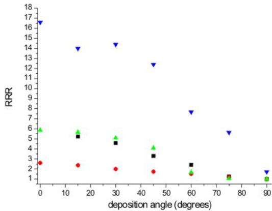
FIG. 8. RRR vs. deposition angle for samples at different level of contamination
