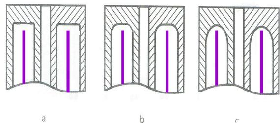
FIG. 3 section view of three QWR. The different curvature radius of the top plate modifies limiting arrival angles.
