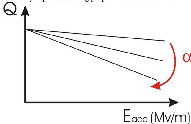
FIG. 1 Q-decaying increasing at high accelerating fields when deposition angle  $\alpha$  increases.
