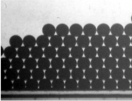
FIG. 17. simulation of film growth at target – substrate angle of 0 degrees
