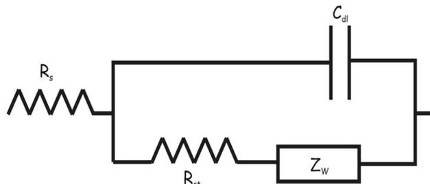
FIG. 14. Equivalent circuit for a porous electrode
