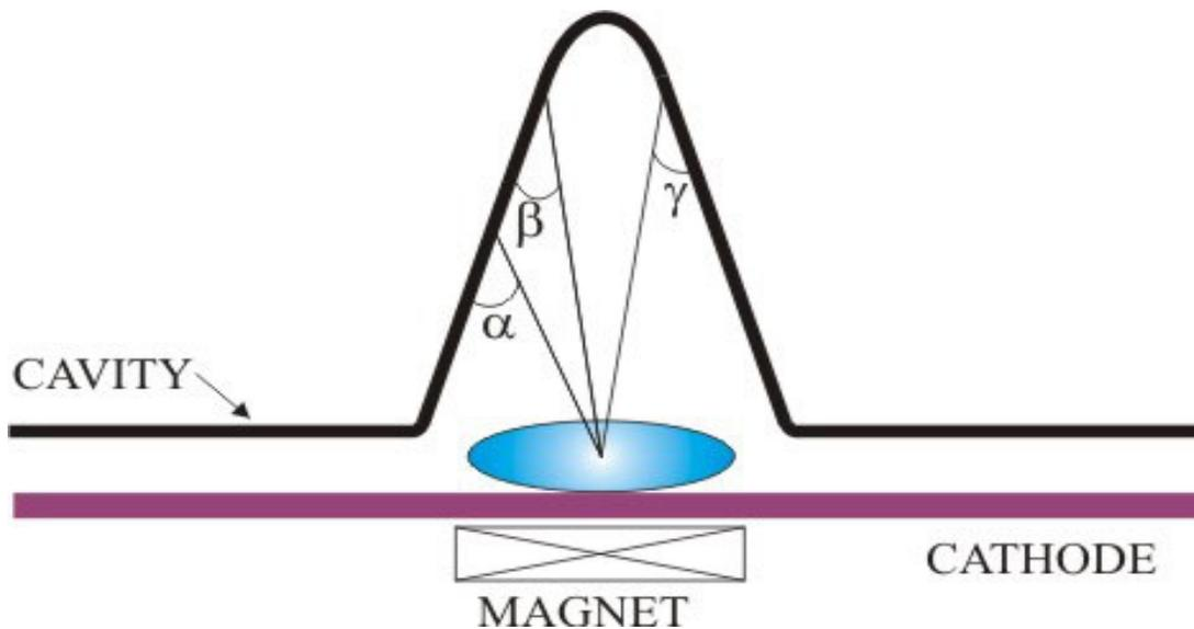
FIG. 5 Arrival angle of niobium atom in different position on the inner surface of a cavity. Also the target-substrate distance is varying.
