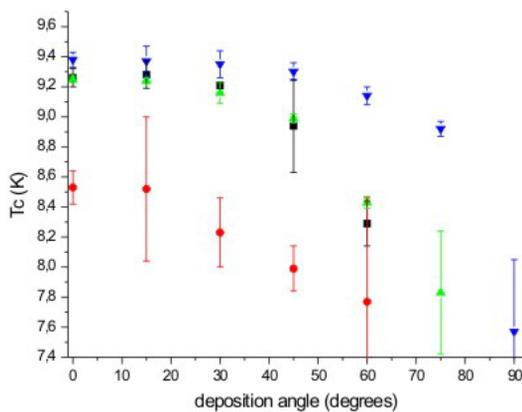
FIG. 9.  $T_c$  vs. deposition angle for samples at different level of contamination
