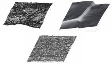
Figure 6: 3D view of annealed samples polished with FNS (top left), FNP (top right) and EP (bottom) (step width 1  $\mu\text{m}$ , vertical scale 25  $\mu\text{m}$ ). The surface topography of only one grain exhibits only a light undulation.
