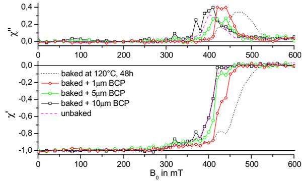
Figure 5: The ac susceptibility of baked BCP-samples after additional chemical etching.
