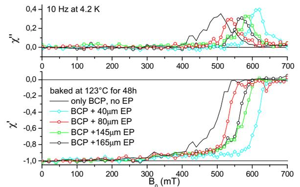
Figure 7: The ac susceptibility of electropolished samples after baking at  $123^\circ C$  for 48 hours.
