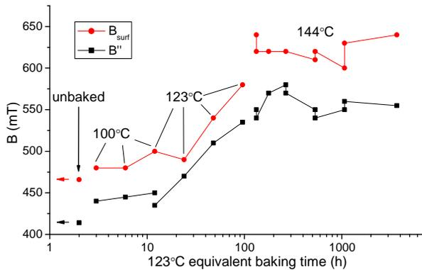
Figure 4: The surface critical field  $B_{surf}$  and the field  $B''$  where  $\chi''$  assumes its maximum, plotted against the equivalent baking time at the reference temperature of  $123^\circ C$ .
