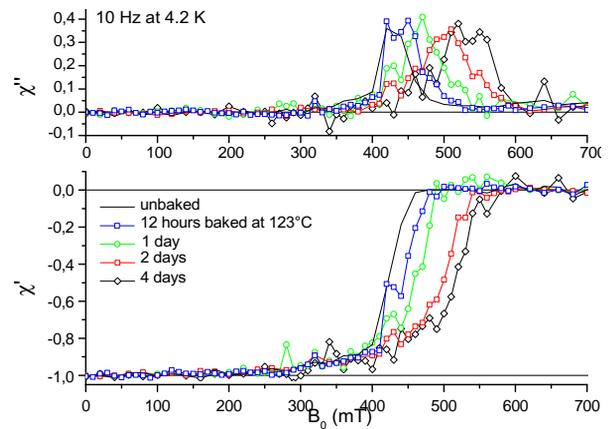
Figure 3: The ac susceptibility of one unbaked BCP-sample and of four BCP-samples baked at  $123^\circ\text{C}$  for times between 12 and 96 hours.
