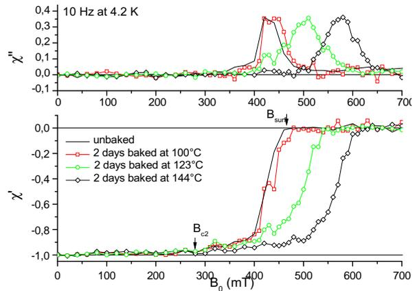
Figure 2: Imaginary ( $\chi''$ ) and real part ( $\chi'$ ) of the ac susceptibility of an unbaked sample and three samples baked for 48h at different temperatures. The values  $B_{c2}$  of the bulk material and  $B_{\text{surf}}$  are indicated for the unbaked sample.
