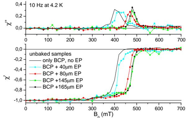
Figure 6: The real and imaginary parts of the ac susceptibility of electropolished samples in comparison with an unbaked BCP-sample.
