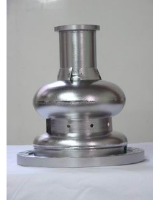
Figure 3: Picture of the 1+1/2 cell cavity.
