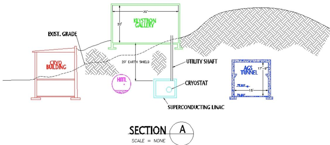
Figure 7: Cross-Section of Enclosures of the BNL-AGS Facilities
