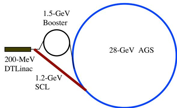
Figure 1: BNL Accelerator Facility and AGS Upgrade
