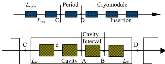
Figure 4: Sequence of Cryostats and Insertions
