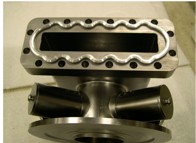
Figure 6: FPC flange Al_{55}Mg “serpentine” gasket.
