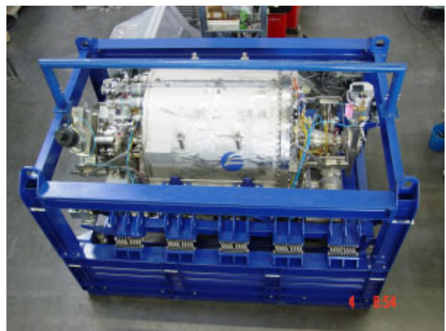
Figure 5: Completed 500 MHz module installed into shipping frame.
