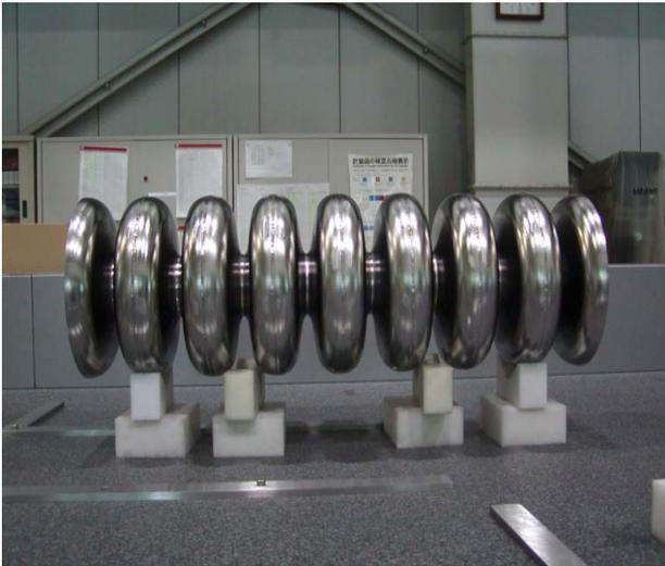
Figure 3: A welded center-cells.
