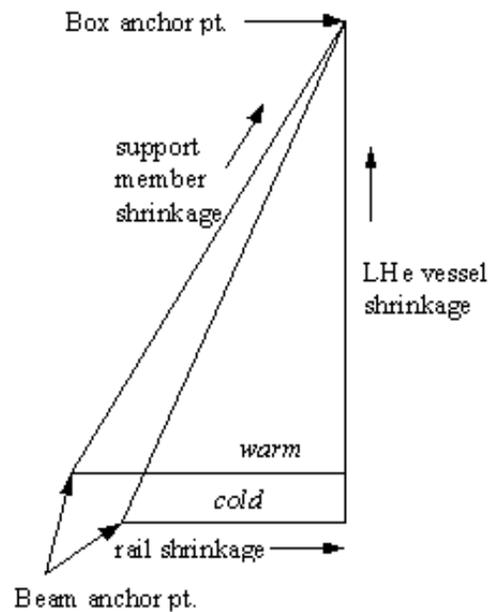
Figure 4: Support geometry.
