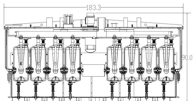
Figure 2: RIA drift-tube cavity cryomodule.
