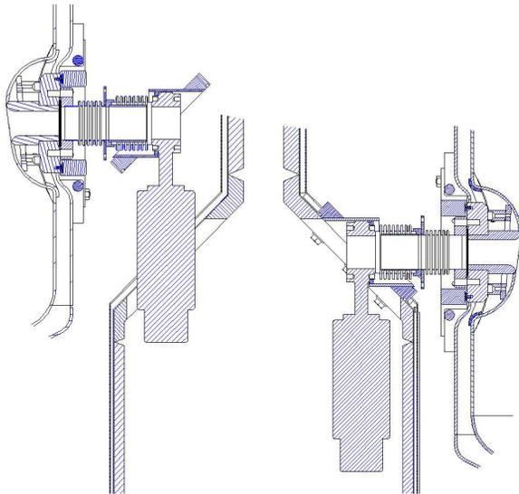
Figure 3: Module-to-module interface showing beam line warm-to-cold transitions, valves, angled vacuum box end walls and module top-loading.
