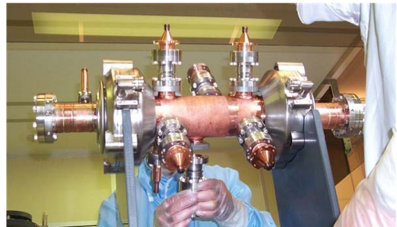
Fig. 1: SUPER-3HC cavity during assembling at CEA.
