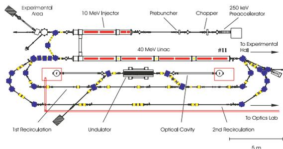
Figure 1: Layout of the S-DALINAC
