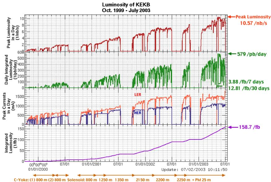
Figure 1: Performance growth of KEKB: peak luminosity, daily integrated luminosity, beam currents of LER (red) and HER (blue) and total integrated luminosity. Bottom arrows shows the total length of a LER beam duct covered by solenoid coils for suppressing the electron-cloud instability.
