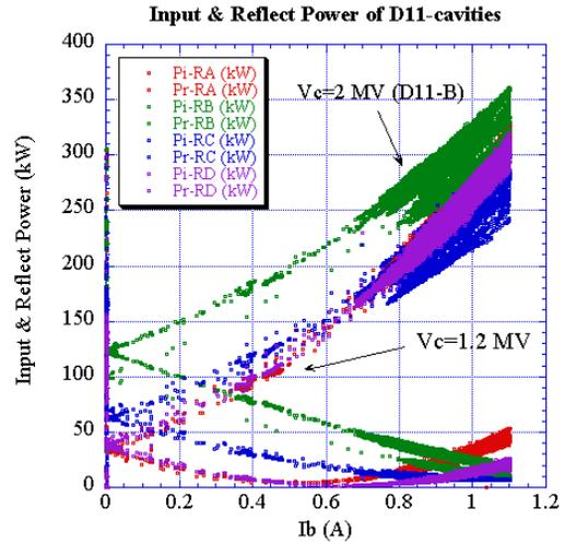
Figure 5: Coupler power of D11-cavities vs. the beam intensity ( $I_b$ ) of HER. One of the D11 cavities (D11B) was operated with the voltage of 1.6 MV, 1.8 MV and 2 MV as a performance test. No degradation of the trip rate was observed.
