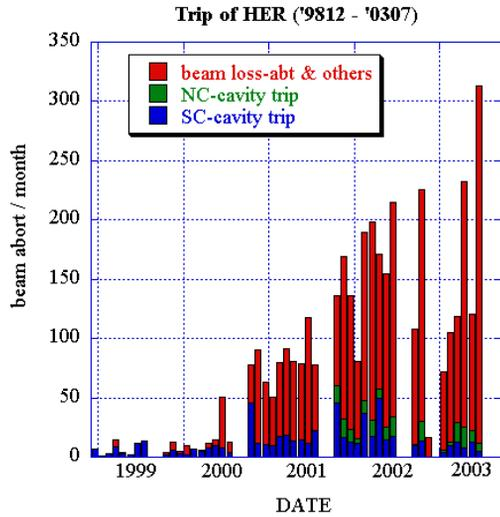
Figure 4: Total trips of KEKB-HER. The number of trips is increasing as the beam intensity improved, however, trips due to RF have never been affected by the intensity.
