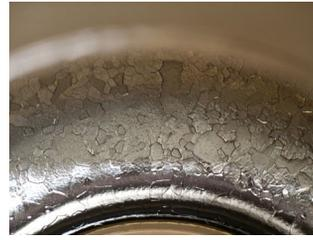
Figure 7b: Picture of the inner surface of C1-15 (no residual Q-slope after baking).
