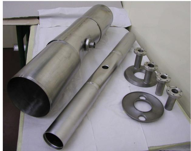
Fig. 4: Nb parts of a HWR, courtesy of ZANON S.P.A.
