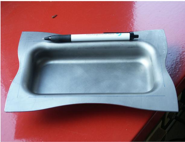
Figure 5: High pressure hydroforming of 230x160x2mm<sup>3</sup> niobium sheet, depth: 30mm, 10mm bending radius.
