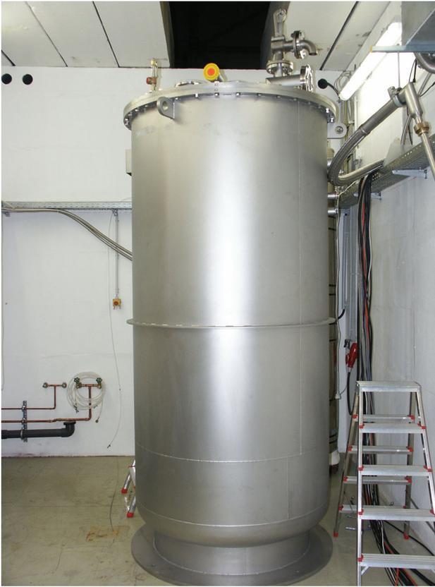
Figure 8: Vertical bathcryostat.
