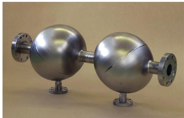
Figure 2: Fixed coupling cavity Built and tested at CERN.
