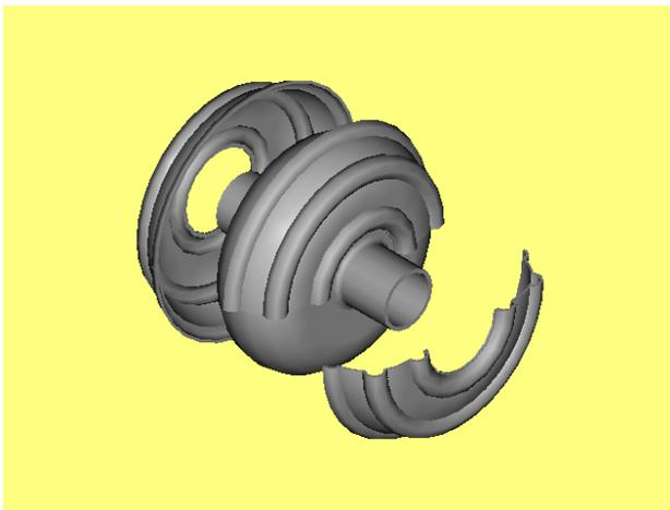
Figure 7: Exploded view of the pipe cooled cavity.
