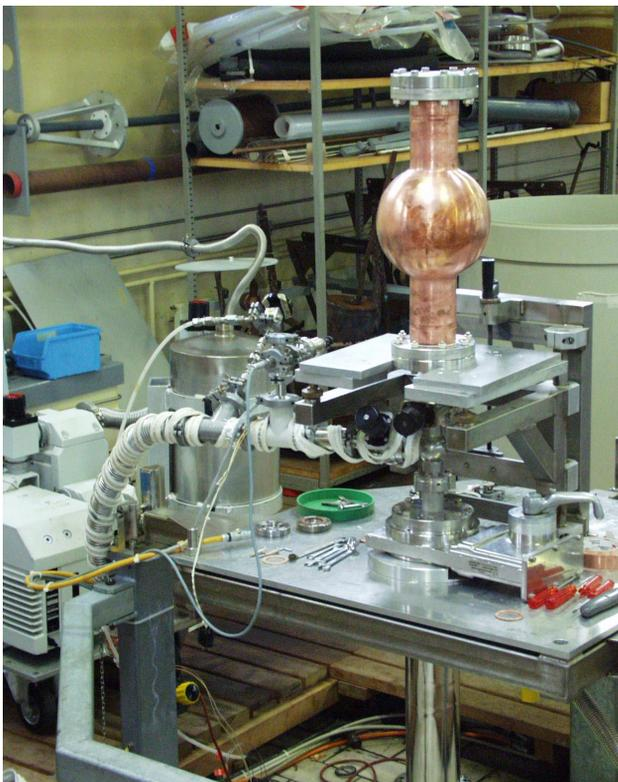
Figure 4: Prototype sputtered single cell cavity. The cavity was built by Spinning In LNL (V.Palmieri) and coated at CERN.
