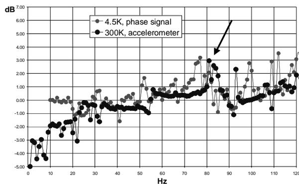
Figure 1: Mechanical response of the  $\beta=0.7$  cavity to longitudinal excitation: the main resonance, pointed by the arrow, is around 77 Hz at 4.5K (81 at 300K).
