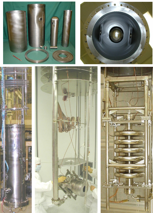
Figure 4: Top: parts for 80.5 MHz QWR (left) and inside view of completed cavity (right). Bottom: 80.5 MHz QWR (left), 322 MHz HWR (middle) and 805 MHz 6-cell (right) on their RF test stands.
